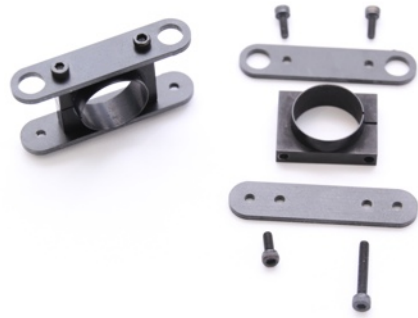
Assembled main tube clamps with G10 composite plates and three M3x6 and one m3x20 screw (each clamp)
